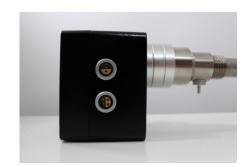
Oxygen probes for measuring the oxygen partial pressure in furnace atmospheres. Suitable for carburizing amtospheres, carbonitriding and endothermic gas generators
