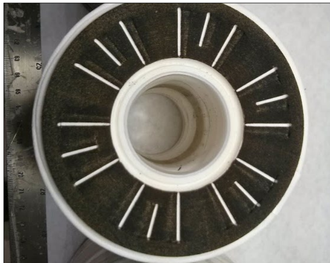
Filter “Dirty Natural Gas”
