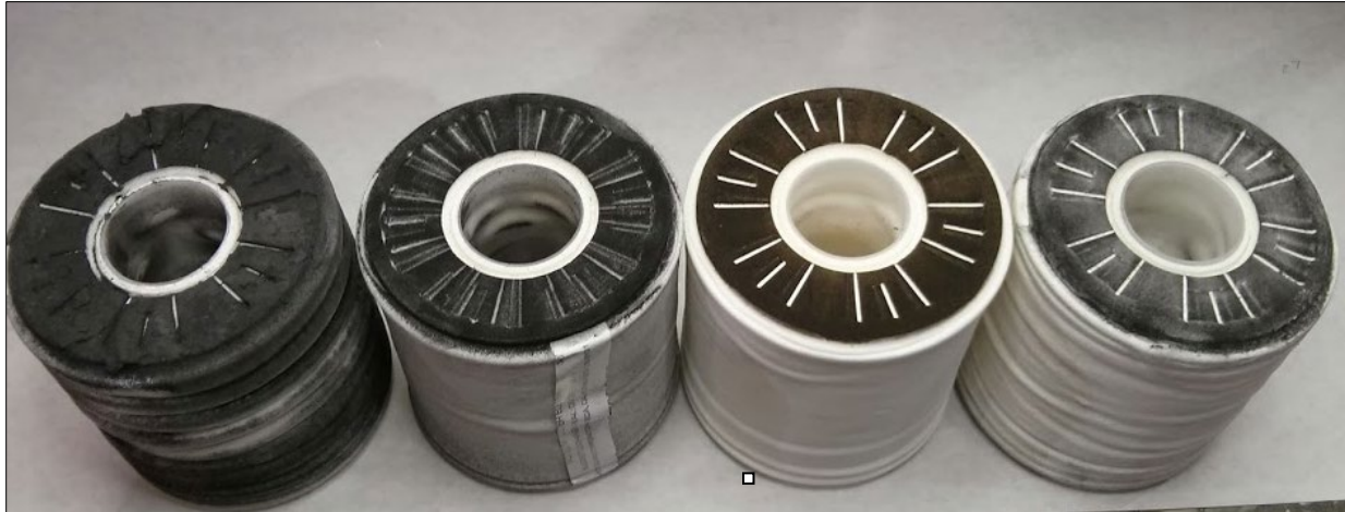
Filters in various stages of contamination
