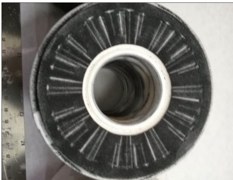
Multiple Indentations from Filter Housing
